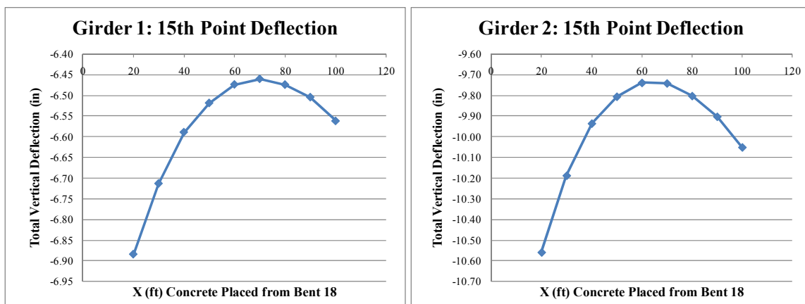
Figure D.13: Total Deflected with Varied Deck Placement Sequence for Girders 1 & 2
