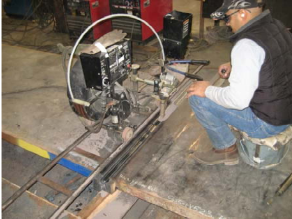
(a) Submerged Arc Weld of Flange Plates
