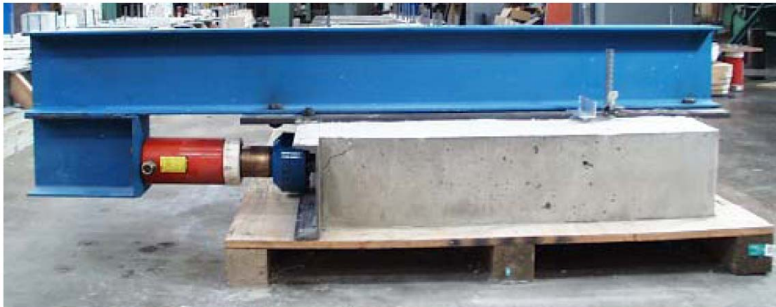
Figure 4.14: Picture of Push-out Test Setup (Topkaya 2002)
