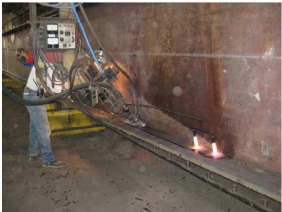
(c) Welding of Flange to Web
