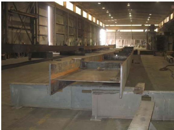
(d) Layout of Two Segments to be Curved
